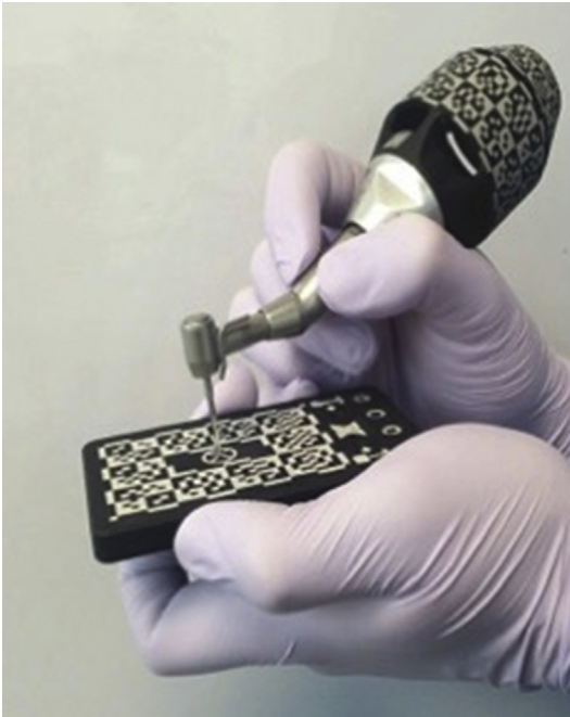
Fig. 7. An implant drill bit is placed on the handpiece and the implant drill bit is placed on the Go Plate perpendicular to the center target. (Courtesy of X-Nav Technologies, Lansdale, Pennsylvania.)
